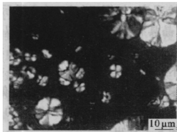
Fig. 8 Polarized optical micrograph of positive four-sectional spherulite Crystallized at 255^{\circ}\text{C} for 20 min
